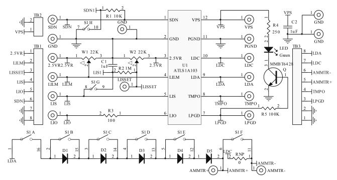
Figure 7. Schematic of ATLS1A103DEV1.0
